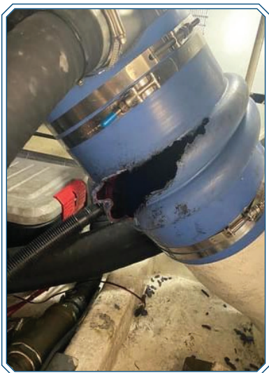
Muskrat enters exhaust pipes, chews through the silicone bellows!
