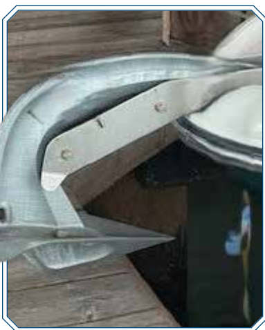
Anchor Extending over Dock is a Trip Hazard
